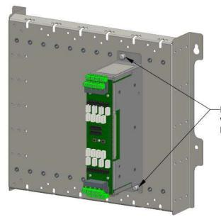
Mount Relay Module with two M6 x 10 Screws provided with module.
